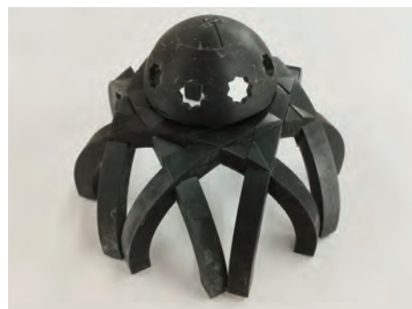
Figure 9: Complete model with interlocked arches and upper dome. Picture of the 3D printed model.
