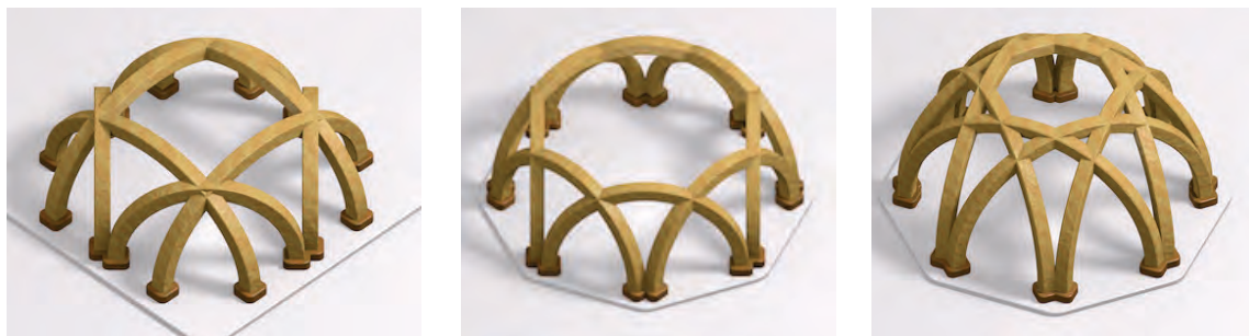
Figure 5: Rendering of the 3 types of ribbed domes: lattice + diamond, and stars [8/2] and [8/3] .
