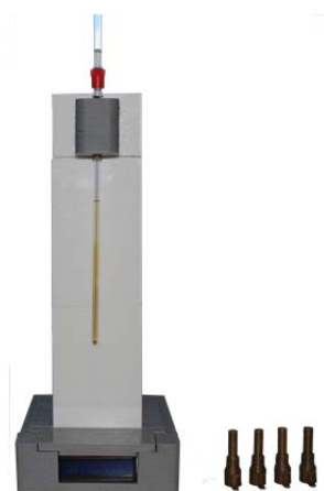
Figure 1. Programmable device for the uniform rotation of NMR tubes.
