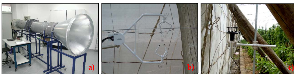
Figure 1. Low velocity wind tunnel designed at the University of Almería (a). 3D (b) and 2D (c) sonic anemometers.
