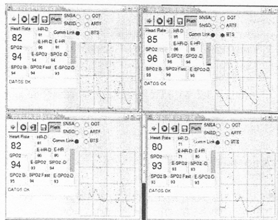
Figure 5. Monitoring screen for a piconet with four SPO2 sensors
